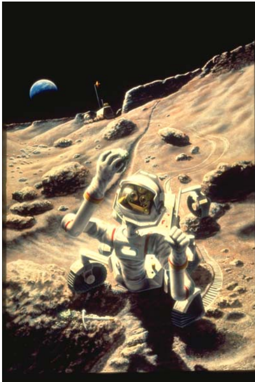
Figure 2. A telepresent robot might extend human “reach” into hostile or remote environments 12 . In this concept, the robotic rover with very high resolution vision and tactile feedback is under the direct and instantaneous control of a human operator at a remote site, thus fooling the human into thinking that they are “present” at the remote locality. This would enable true field study on the planets by melding a human mind with a robotic body. Such techniques can be evaluated on the Moon.
